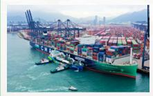
YANTIAN delivered liquefied natural gas ("LNG") bunker fuel via ship-to-ship transfer in its first LNG bunkering operation in South China. Currently, it has the world's largest LNG bunker vessel fitted with Type C tanks¹.
