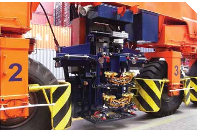
YICT converted a large percentage of its diesel-driven RTGCs into electricity-powered ones
